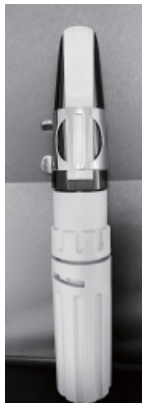
Figure2. Clarinet Mouthpiece and Silencer (Front)
