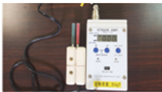
Fig.1 A hand dynamometer for infant. (T.K.K.1269r)
